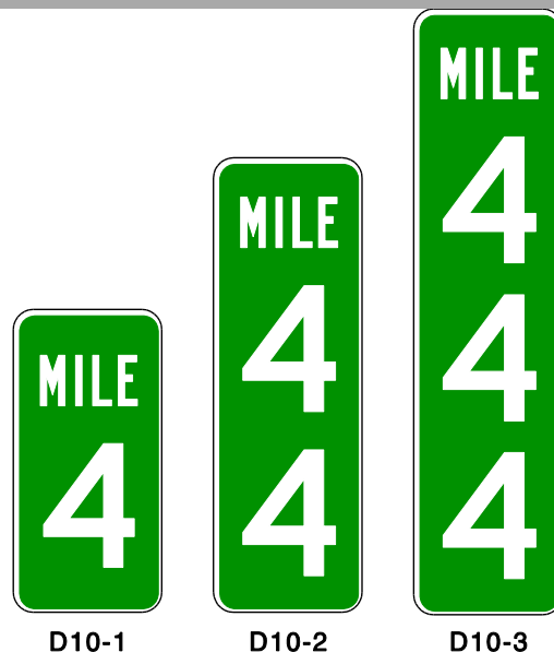
Figure 2H-2. Reference Location Signs*
