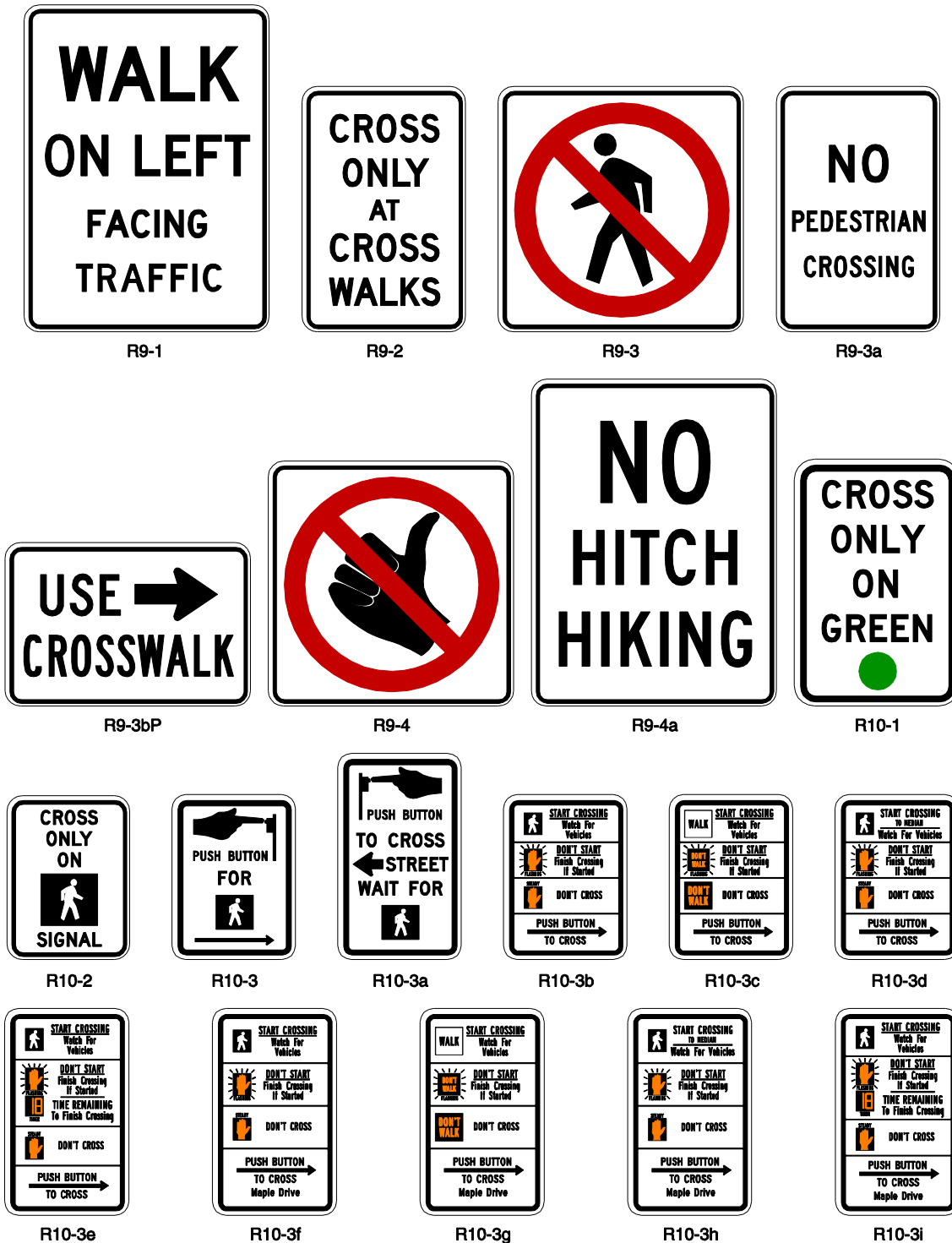
Figure 2B-26. Pedestrian Signs and Plaques (Sheet 1 of 2)
