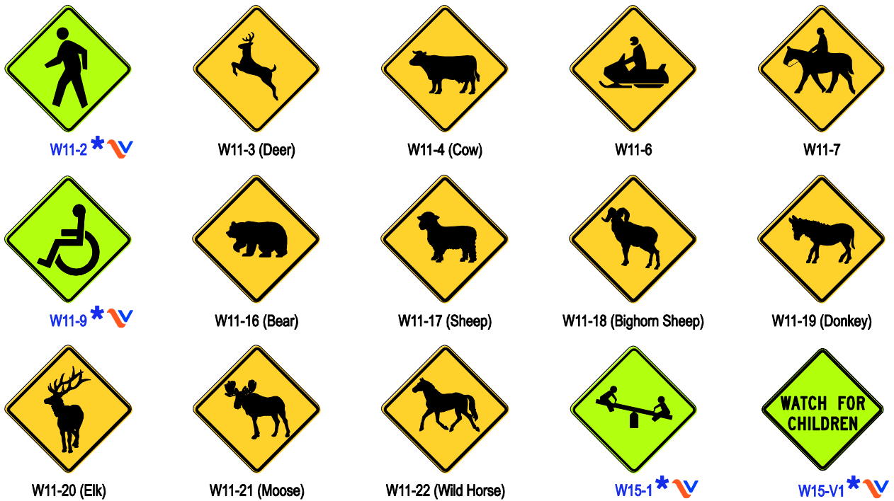
Figure 2C-11(VA). Non-Vehicular Warning Signs
