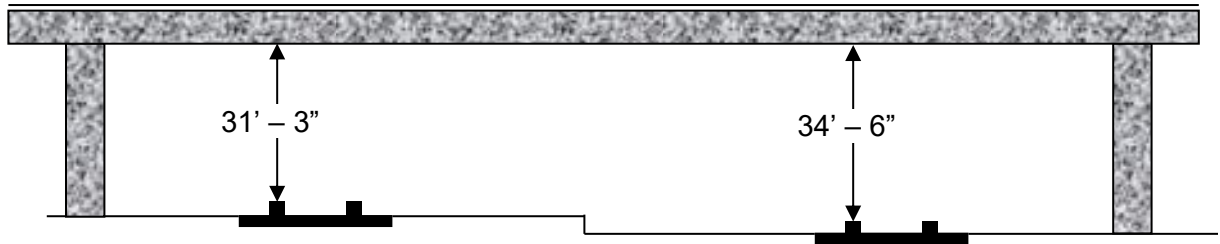
Railroad 31'- 3" beneath structure
