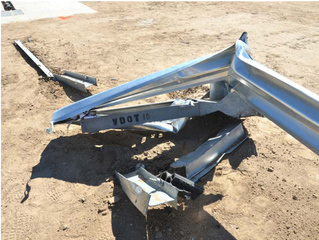
FIGURE 36. Test Article Damage
