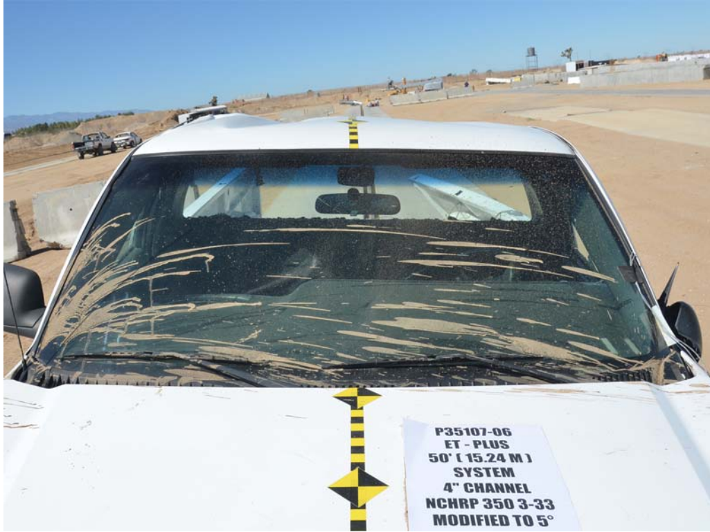
FIGURE 51. Post-Test View of Windshield
